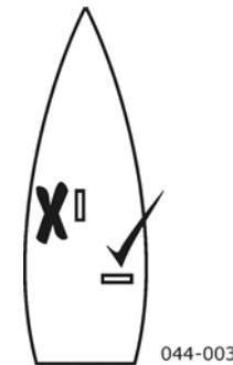
*For optimum signal avoid mounting the transmitter on a longitudinal surface*
